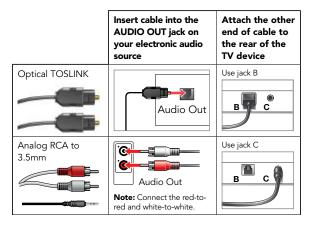
**Tip:** During initial setup, a solid blue LED confirms the audio cable is properly attached to the TV device and audio streaming is active.
